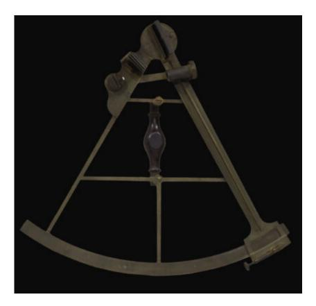
14.5 inch radius vernier sextant by Jesse Ramsden, constructed in brass, signed on the lower cross bar Ramsden London, scale divided to 130o direct to arc, vernier inscribed G. Vancouver, braced index arm, index mirror with Maskelyne flap, sighting tube, four shades, secondary mirror on rearmounted adjusting lever, wooden handle and brass pin feet, lacking secondary mirror and part of sighting tube.
