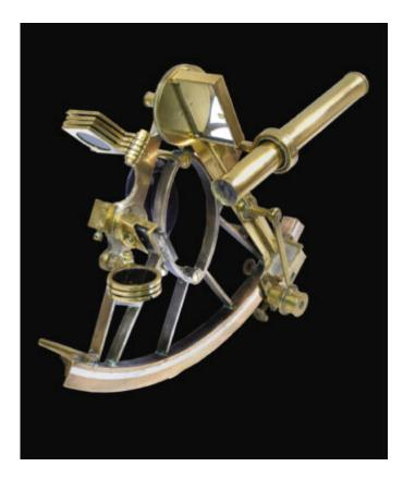
7 inch radius sextant, lattice frame with silver scale 0-150° and vernier, seven shades, telescope, wooden handle, in fitted case.
